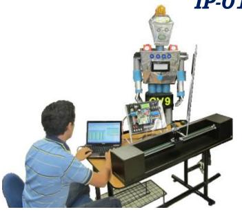
The inverted pendulum is an excellent lab practice for those interested in control, systems, mechanics, process, electronics, mechatronics and robotics. This is a very fundamental application for robotics to understand among other concepts, the equilibrium concept.
